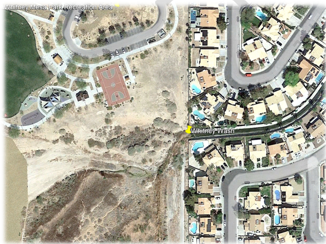
Figure 12. Whitney Mesa Park and Whitney Wash (Whitney Drain), showing channelized, concrete-lined wash routed through subdivision. (Snippet from Google Earth.)
