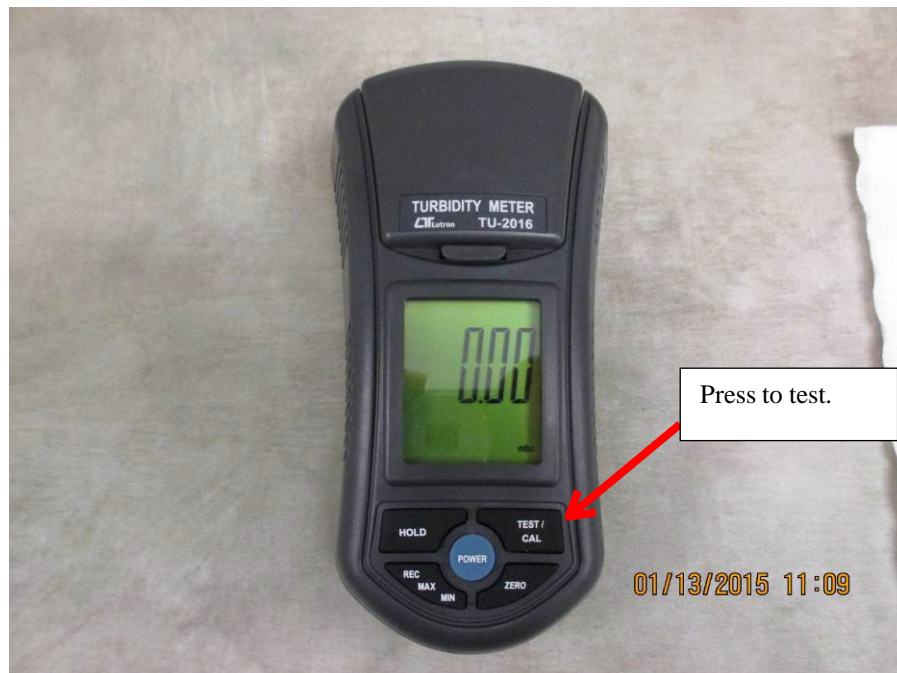
5 - Sample Reading of DI H 2 O (0 NTU)
