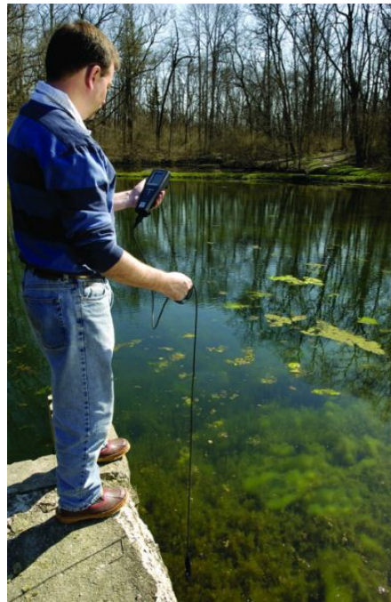
10 - 3 rd Option - Measure D.O. in a Pond
