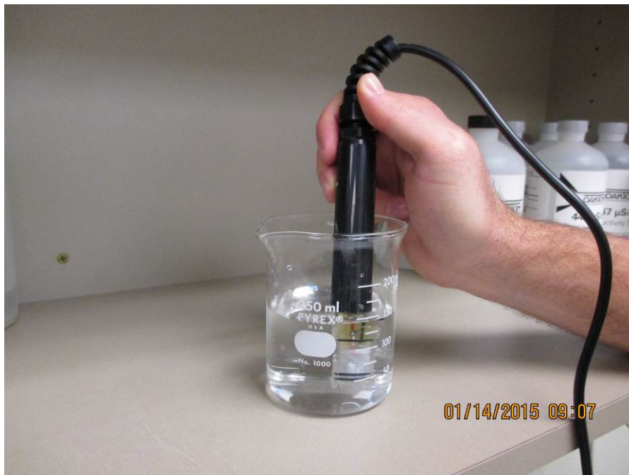
8 - 1 st Option - Measure D.O. in a Sample Beaker
