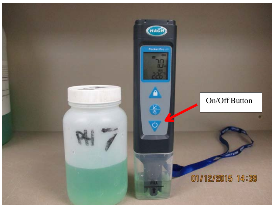
4 - Sample Measurement (solution of 7.0 pH)
