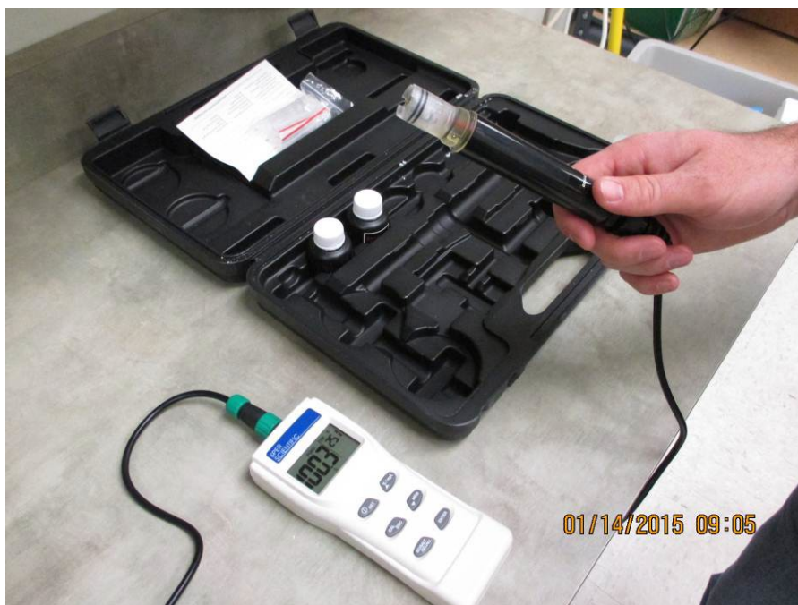
5 - Pre-Calibration (waiting for stable value)
