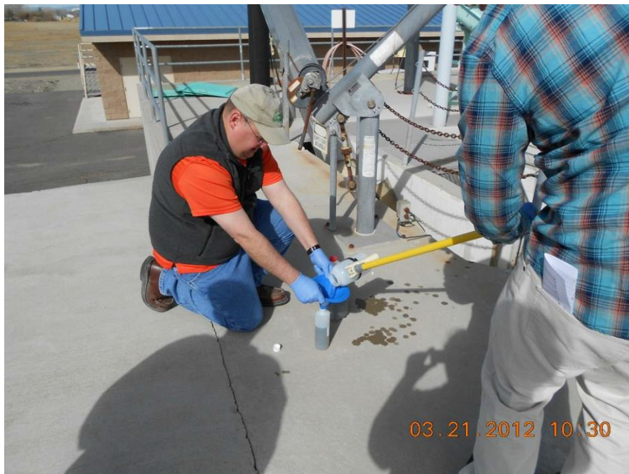
Fig. 14 - Filling a Metals Bottle with a Funnel
