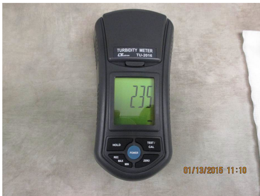
6 - Sample Reading of Turbid H 2 O (e.g. 235 NTU)
