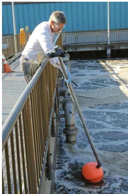
13 – Example of a “Fixed” Reference D.O. Sensor
