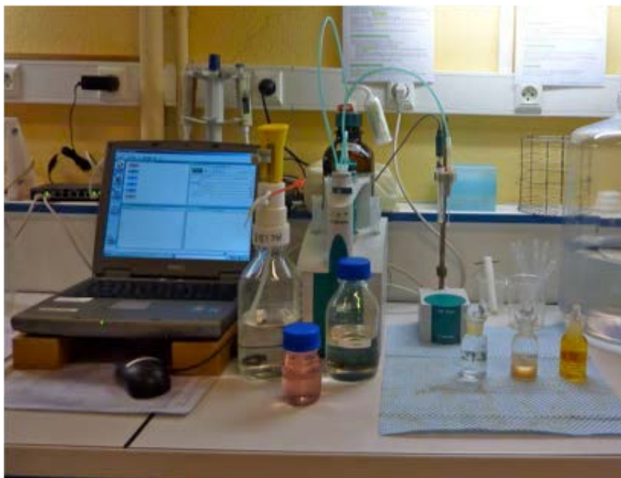
14 - Lab Reference Winkler Method
