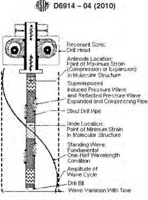
FIG. 1 General Principle of Sonic Drilling
