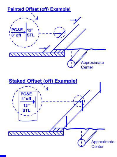
4 An operator's identifier (name, abbreviation or initials) is to be placed at the beginning and at the end of the proposed work. In addition to the previous, subsequent operators using the same color, will mark their company identifier at all points where their facility crosses another operator's facility using the same color. The maximum separation of identifiers is to be reduced to a length that can be reasonably seen by the excavator when the terrain at the excavation site warrants it.
