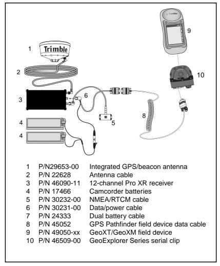
To use a GPS Pathfinder Pro XR receiver with a Trimble GeoXT or GeoXM, connect the system as shown in Figure 5.6.
