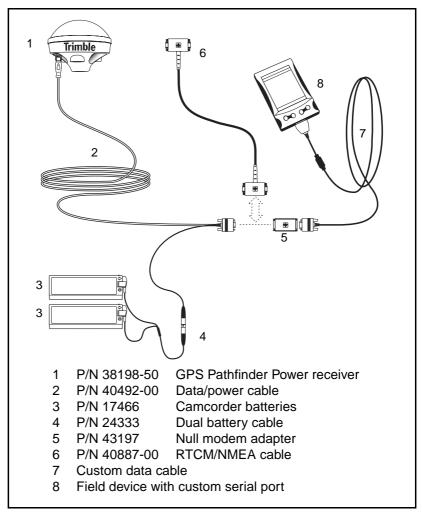
Figure 5.13 GPS Pathfinder Power receiver / field device with custom serial port connection diagram
