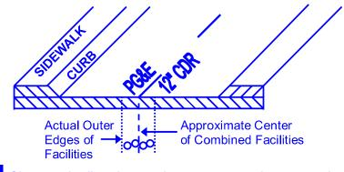
3 Changes in direction, and lateral connections are to be clearly indicated at the point where the change in direction or connection occurs with an arrow indicating the path of the facility. A radius is indicated with marks describing the arc. When providing offset markings, (paint or stakes), show the direction of the facility and distance to the facility from the markings.
