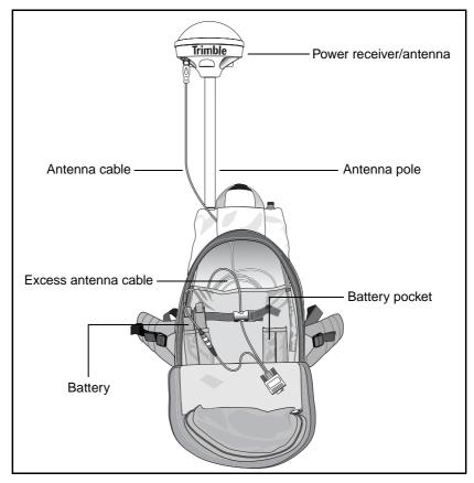
Figure 5.15 GPS Pathfinder Power receiver in the backpack
