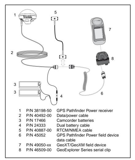
To use a GPS Pathfinder Power receiver with a Trimble GeoXT or GeoXM, connect the system as shown in Figure 5.12
