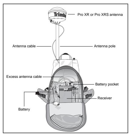
Figure 5.14 illustrates the features inside the backpack.
