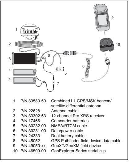
To use a GPS Pathfinder Pro XRS receiver with a Trimble GeoXT or GeoXM, connect the system as shown in Figure 5.9.
