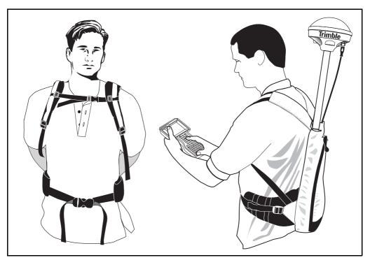
Figure 5.16 Backpack adjustment front and back views
