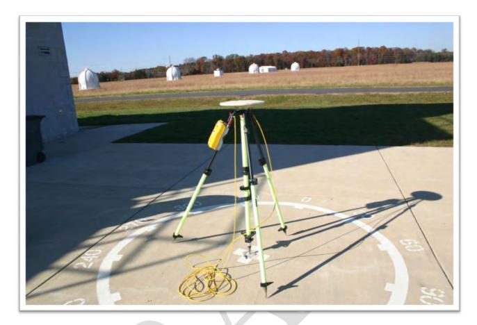
Figure 2. Trimble GPS Receiver on GPS Antenna Tripod
