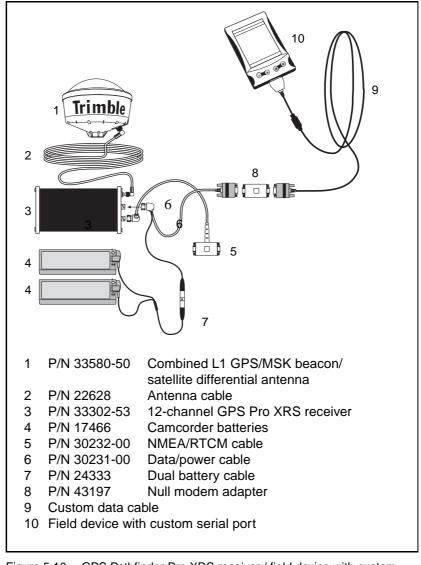
To use a GPS Pathfinder Pro XRS receiver with a field device that has a customized serial port, connect the system as shown in Figure 5.10.
