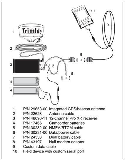
To use a GPS Pathfinder Pro XR receiver with a field device that has a customized serial port, connect the system as shown in Figure 5.7.
