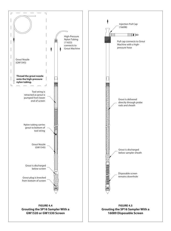
**3.** Place a mark on the extension rod even with the top of the probe rod. Apply downward pressure on the extension rods and push the grout plug out of the screen. The mark placed on the extension rod should now be below the top of the probe rod. Remove all extension rods.
