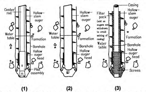
FIG. 2 Sketch Showing Basic Three-Step Procedure for Installation of Subsurface Water-Quality Monitoring Device Using the Hollow-Stem Auger Drilling Method incremental removal of the hollow-auger column as completion materials such as filter pack, annular seals, and backfill are installed as required.
