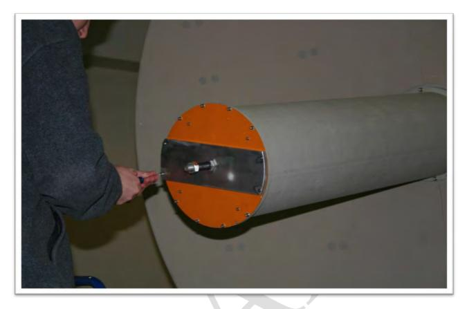
Figure 3. NAGS flush-mount plate on NAGS end
