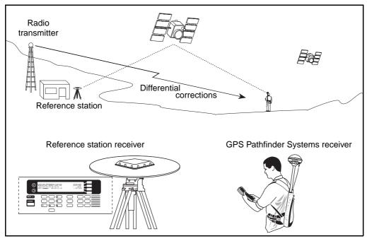
Figure 4.1 Components of a DGPS system
