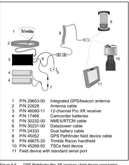
Figure 5.5 GPS Pathfinder Pro XR receiver / field device connection diagram
