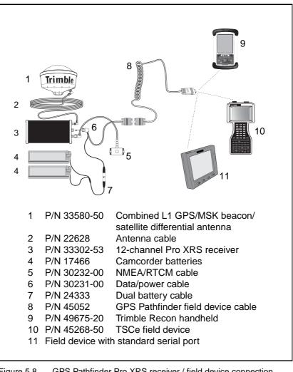
Figure 5.8 GPS Pathfinder Pro XRS receiver / field device connection diagram
