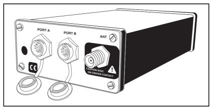
Figure 5.2 GPS Pathfinder Pro XR and Pro XRS receiver back panel
