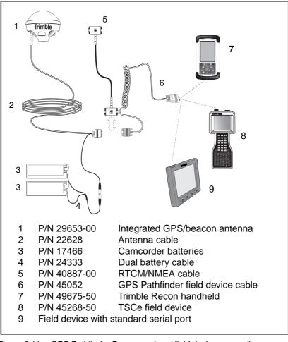
Figure 5.11 GPS Pathfinder Power receiver / field device connection diagram
