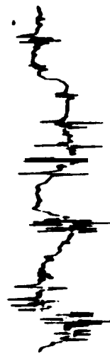
Simultaneous logs Intermittent noise probably caused by drilling equipment of the well
