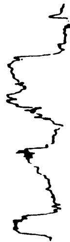
Simultaneous logs Intermittent noise probably caused by drilling equipment of the well
