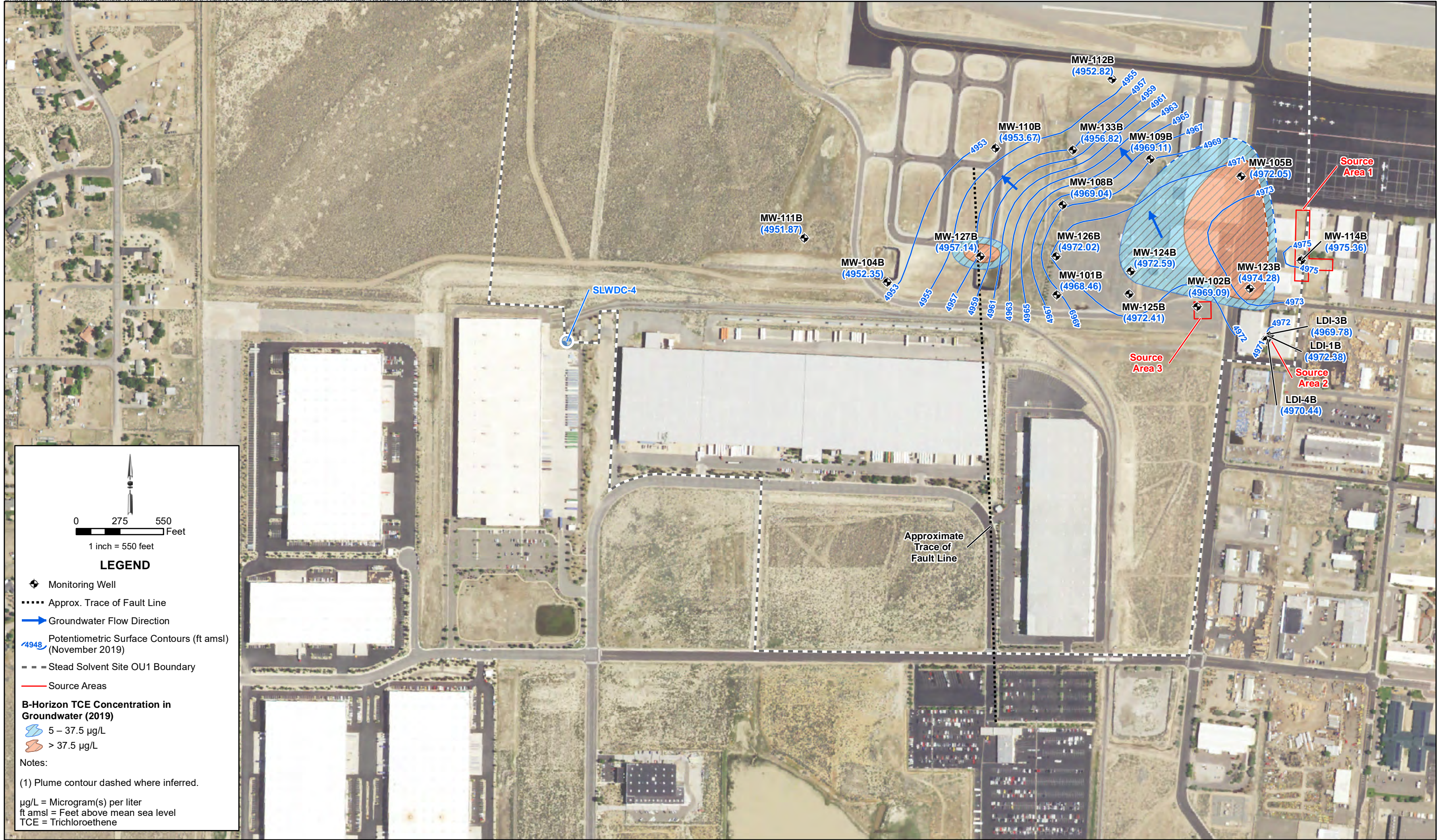
FIGURE 5B4 GROUNDWATER POTENTIOMETRIC SURFACE NOVEMBER 2019 (B-HORIZON) 2019 LONG-TERM MONITORING AND REMEDIATION PROGRESS REPORT STEAD SOLVENT SITE OPERABLE UNIT 1, RENO, NEVADA
