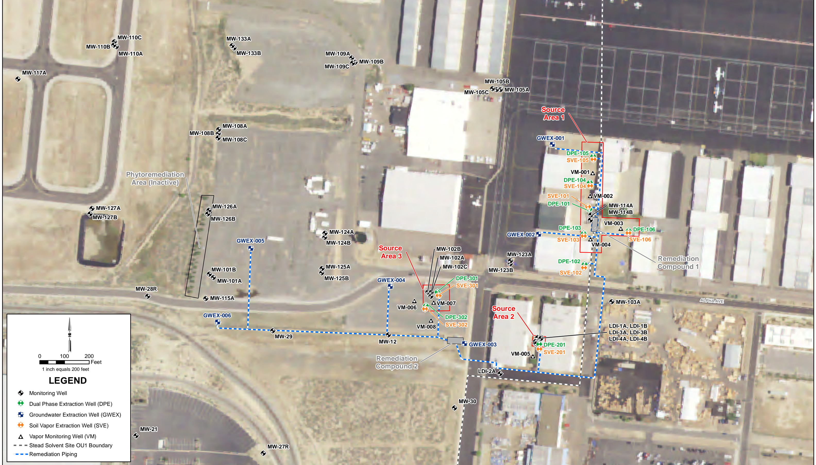
FIGURE 3 SITE PLAN WITH REMEDIAL INFRASTRUCTURE 2019 LONG-TERM MONITORING AND REMEDIATION PROGRESS REPORT STEAD SOLVENT SITE OPERABLE UNIT 1, RENO, NEVADA
