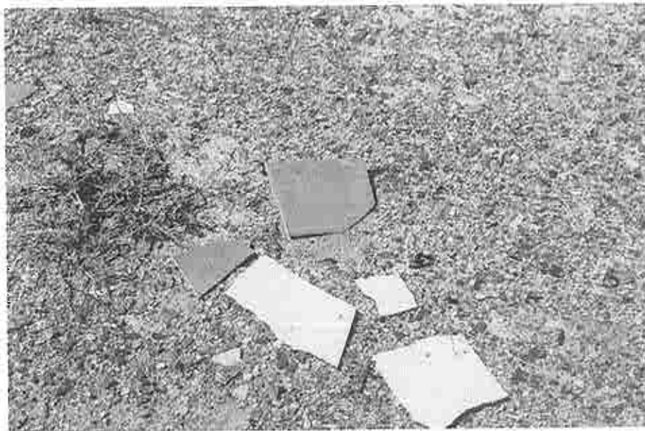
Photograph C-8: Suspect asbestos-containing tiles scattered on the ground at Building 1230 (AC Magazine).
