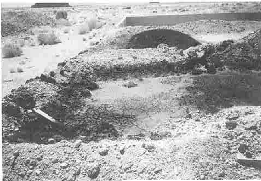
Photograph C-18: View of oil stained soil at oil sludge dumping area from the oil refinery operations being placed on top of a former TAAF building slab foundation.
