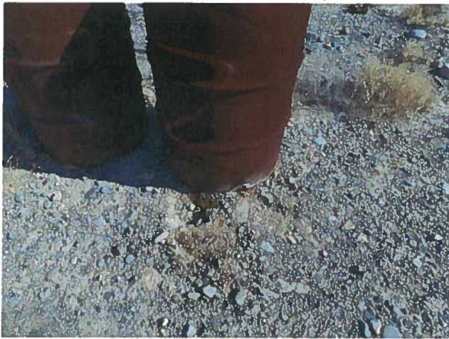
On-site drums (one punctured at base)
