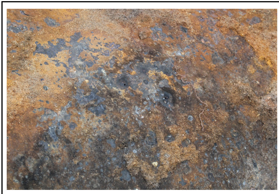
Corrosion damage on heating oil tank
