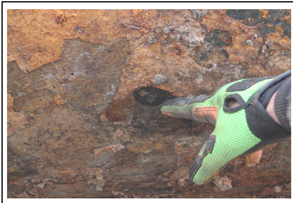
Waste oil tank corrosion damage
