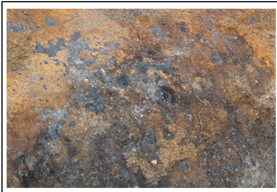
Corrosion damage on heating oil tank
