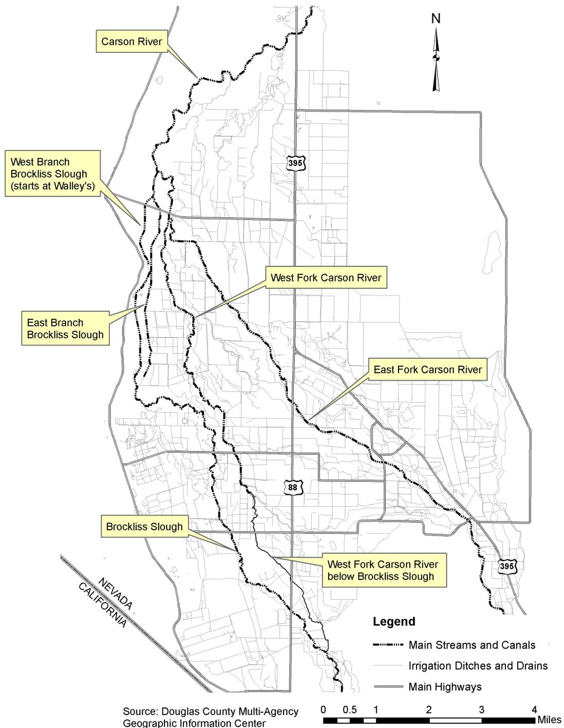
**Figure 5. Main Streams, Canals, Ditches and Drains in Carson Valley**
