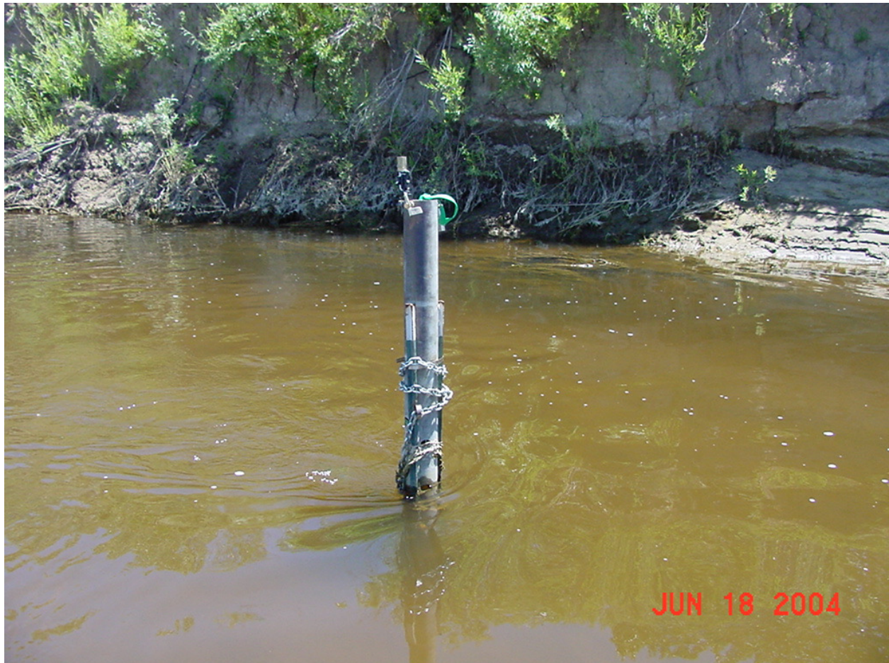
YSI Dissolved Oxygen Monitoring Sonde on the Carson River below Highway 395 (Cradlebaugh Bridge), Photograph by Z. Latham, June 2004
