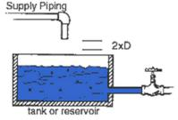
However, an air gap to be used as meter protection (containment) is unusual. If there is the potential for a piping arrangement cross connected with sewage or reclaimed water, the service will need to have an air gap, an RP is not considered sufficient.
