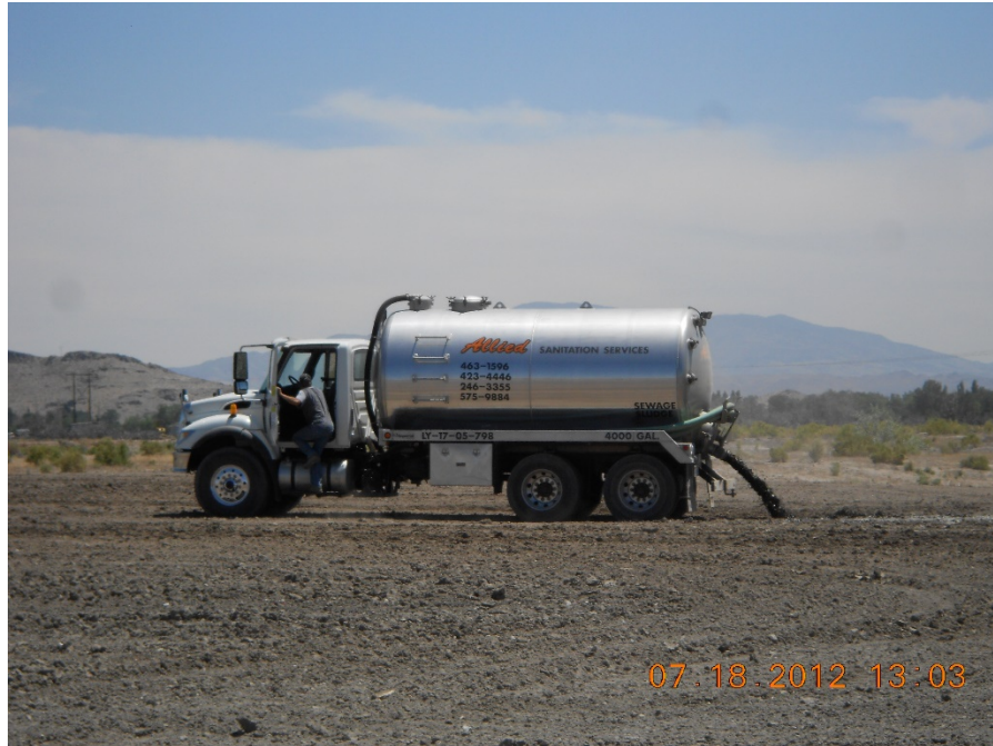
Fig. 2 - Septage application (surface)
