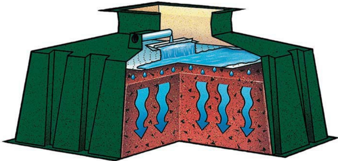
Figure 28-1. Typical peat filter
