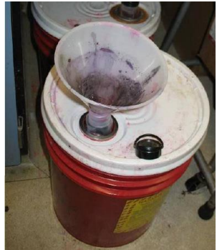
This container is considered “open”. If not actively adding to or removing from the container, remove funnel and close the container.
