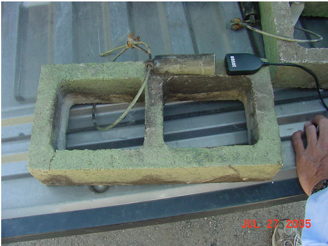
Downloading data from thermograph datalogger
