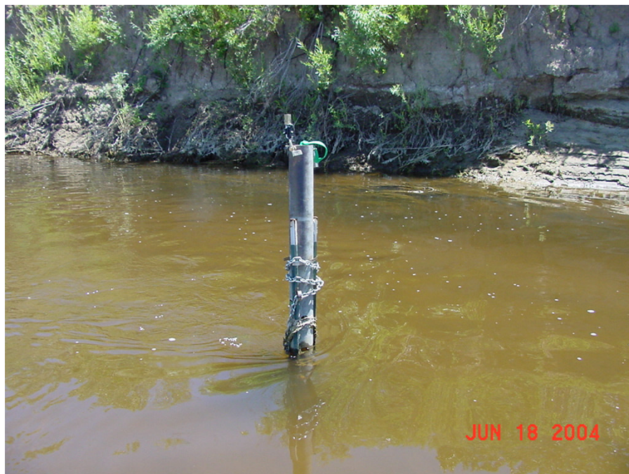
Figure 3. Dissolved Oxygen and Temperature Sonde Deployment by Desert Research Institute – Carson River at Cradlebaugh Bridge (photograph by Z. Latham, 2004)
