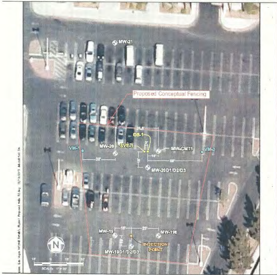
Satellite view of above picture: Overview Map of site work with Potassium Permanganate at 3528/3661 South Maryland Parkway, Las Vegas, NV
