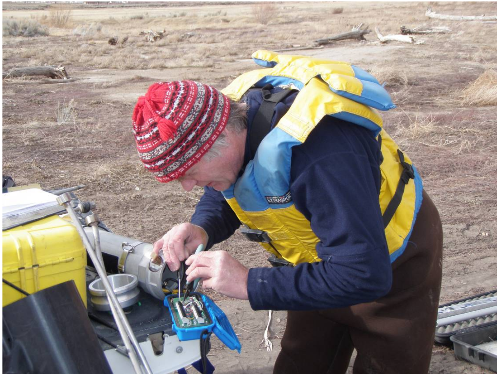
Configuring CR206 data logger to select thermistors. Carson River March 2009.
