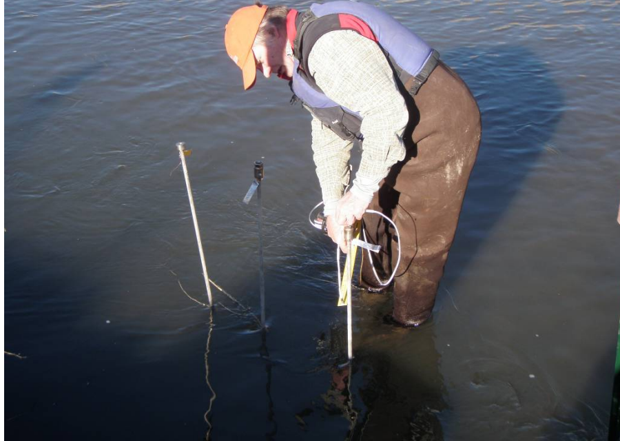
Measuring water level in piezometer with electric sounding tape. West Fork Carson River March 2009.
