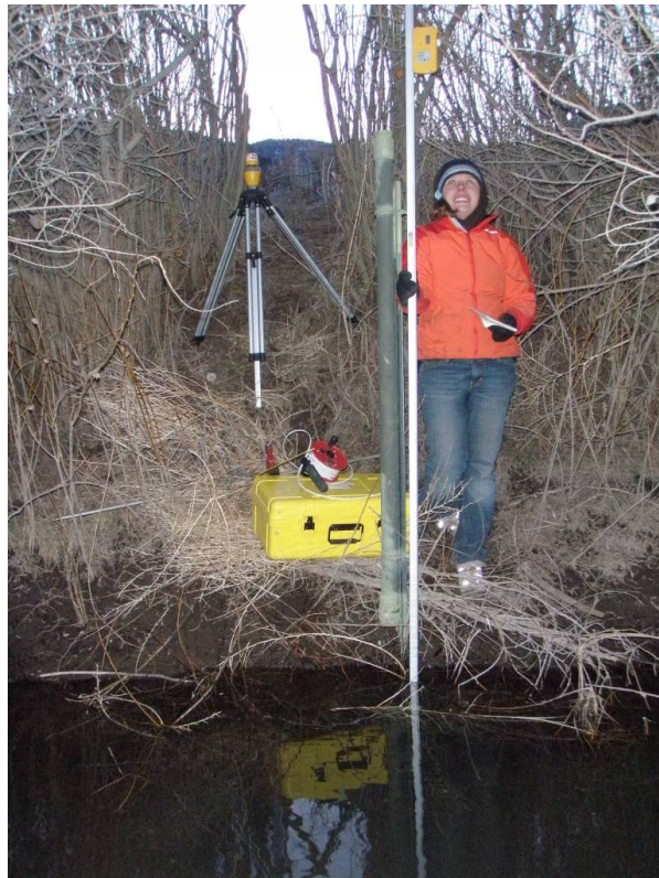
Measuring water level in piezometer with electric sounding tape. West Fork Carson River March 2009.
