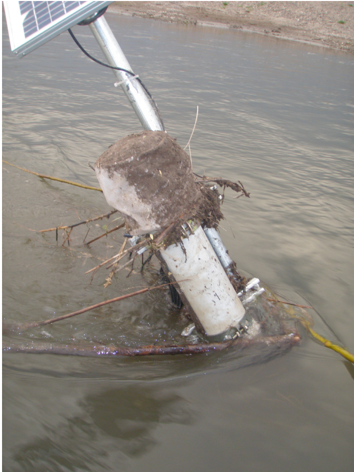
Submersible Caretta vault used to protect data logger East Fork Carson River May 2009. Complete data records of bed temperature profile were collected during the runoff flows at these stations. The white mast is a radio antenna that allows data to be retrieved from shore.
