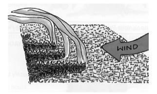
Use an ignition device that does not produce black smoke, such as butane, propane or diesel oil burners. A burning tire is a poor choice for an ignition device – this method generates excess smoke and is dangerous.
