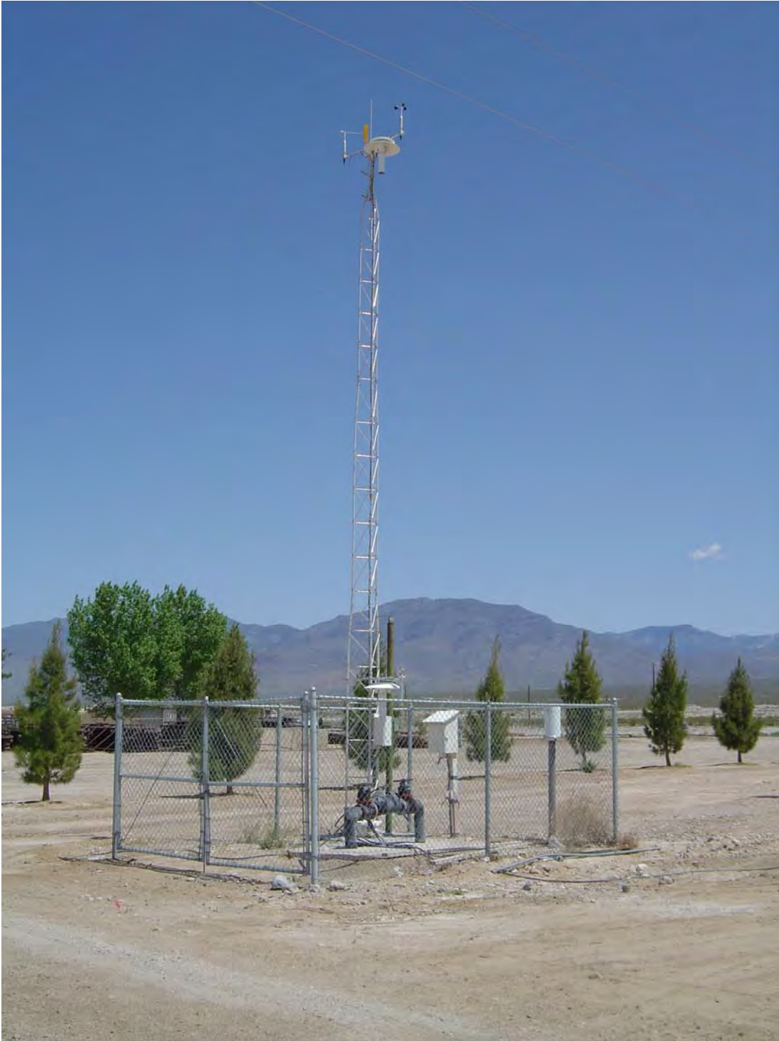
Figure 5. The official 10-meter MET tower to collect meteorological data at the Pool site. Met data will also be collected at each PM_{10} monitor to compare against the 10m tower.
