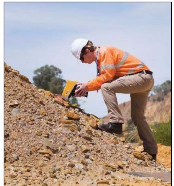
Figure 3: Hand-held soil-metal detector being used to assess the presence of specific metals in soil samples.
