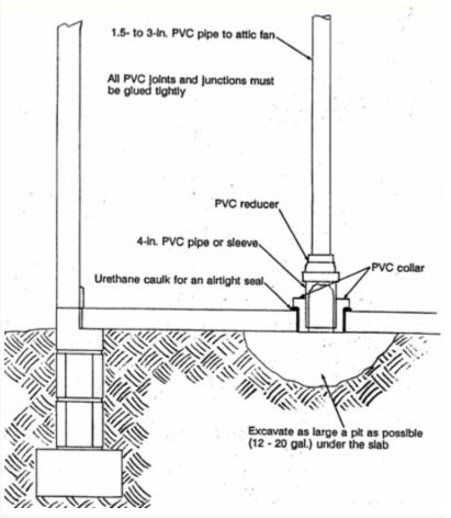
entire footprint of the slab. In these cases, modifications may include installing a bigger fan and/or installing additional sumps to help extend the suction field.
